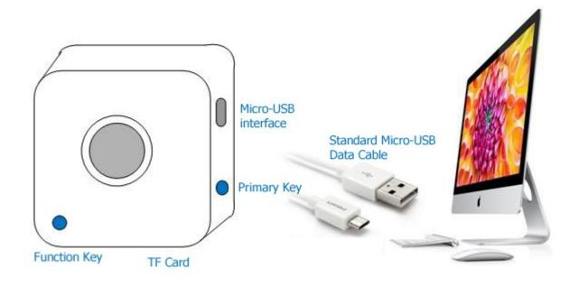
2.After the PC inserts BPI-D1 micro - USB programming cable, the firm programming tools will detect the launch of the application. Once connected, a yellow status bar will appear next to the device in the window, and the status will show "Ready" (please recheck and repeat the steps above if no response). Press the "Start" button on the top to start the firm programming automatically.
