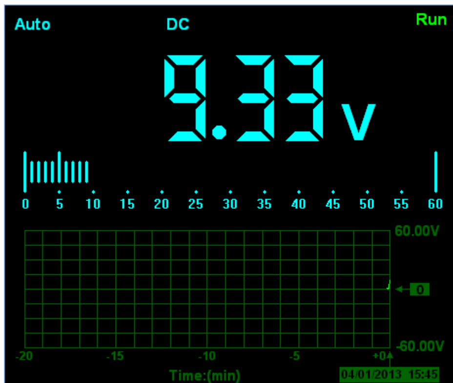
Figure 2-2 DC Voltage Measurement
