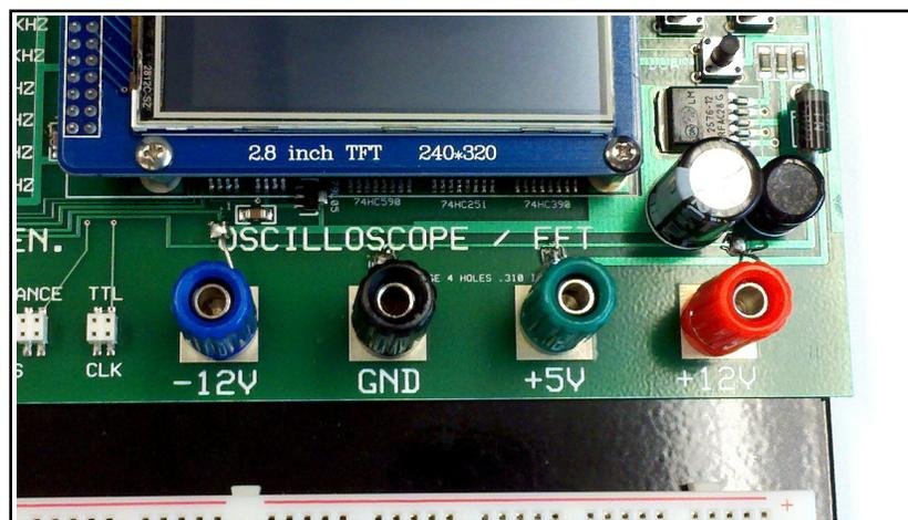
**Figure 4: Bakerboard power supply connections.**
