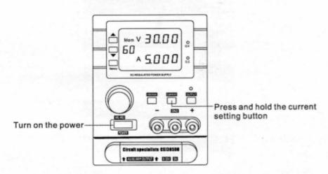
When current protection is set to steady-state current output, set the maximum power supply output to the set current value to protect the power supply device from damage resulting from under-current, and protect the load device from damage due to over-current.
