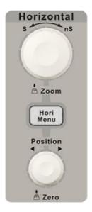
Hori Menu: Press the button to open horizontal control menu under which you can turn on/off the delay sweep function and switch the save modes between "long save" and "normal save".
