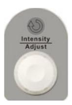
Adjust waveform brightness While the light above the knob is dark, adjusting the knob will change the waveform brightness, which ranges from 30%~100%. Turning clockwise means increase while counterclockwise means decrease. You can also select "intensity" in "DISPLAY" menu and then adjust the knob to change the waveform brightness.
