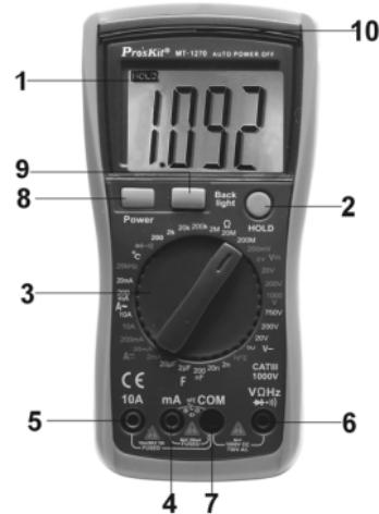
2. If LCD displays “1”, it indicates overload, should turn the knob to the higher range.
