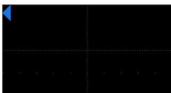
When the trigger position is outside the screen, the direction of the triangle changes to point outside the screen.
