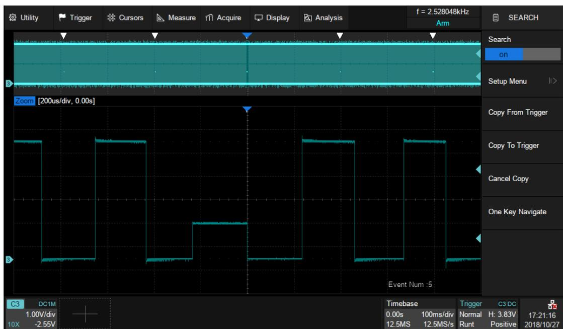
Press the **Run/Stop** button on the front panel to stop the acquisition, and then follow the steps **Navigate** > **Type** to select "Search Event". The following figure
