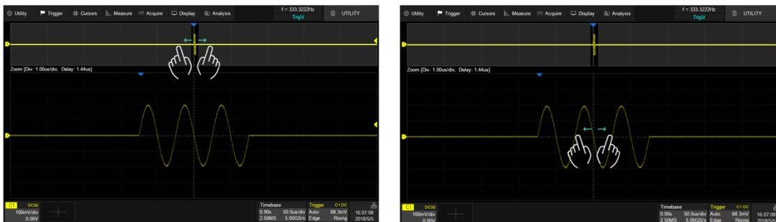
Adjust the horizontal scale of Zoom window by horizontal pinch and spread in the gray area of the main window or in the Zoom window
