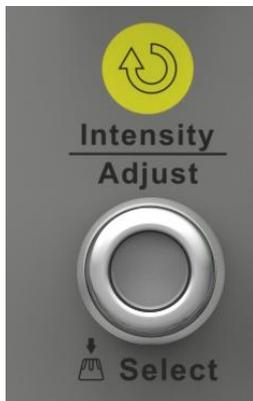
When the parameter setting area is highlighted, you can use the Universal Knob to adjust or set the parameter. Press the knob to select an option from the list.
