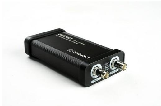
The SAG1021 function/arbitrary wave generator module is capable of generating variant waveforms with frequency up to 25 MHz and amplitude up to  $\pm 3$  V. Users can edit and import arbitrary waveforms using the SIGLENT EasyWave software or import edited waveforms through a U disk.
