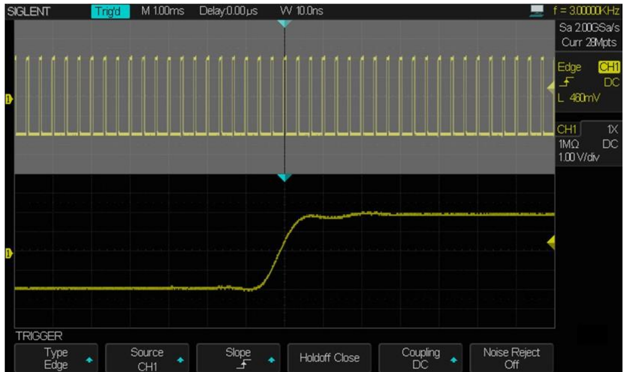
Figure 8 Zoom function in deep memory depth
