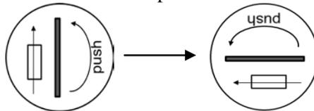
2. If the fuse is fused, please change fuse of same specification based on machine model. See the table blow for matching information of fuse and machine model.
