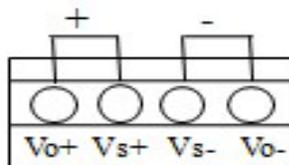
$V_{o+}, V_{o-}$ : output terminals, the same with the rear board output terminals
