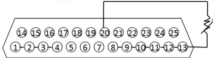
To set the 10V/10K $\Omega$  or 5V/5K $\Omega$  external analog setting range, open the MENU (Menu) → CONFIG (Configure) → Ext-Ctrl (External Analog Control).
