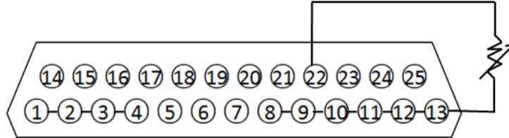
To set the 10V/10KΩ or 5V/5KΩ external analog setting range, open the MENU (Menu) → CONFIG (Configure) → Ext-Ctrl (External Analog Control).
