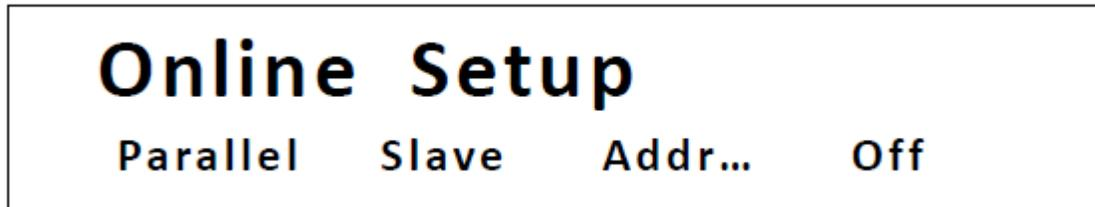
2. While Parallel or Series is flashing, use keys to toggle between the two options. Set to Parallel for parallel connection and Series for series connection.
