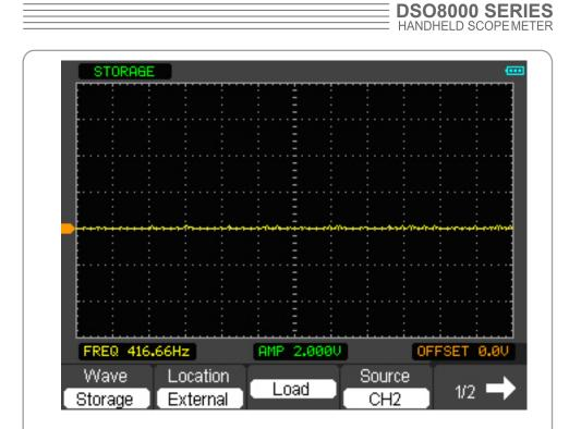
Figure 5-23 The External Waveform Window
