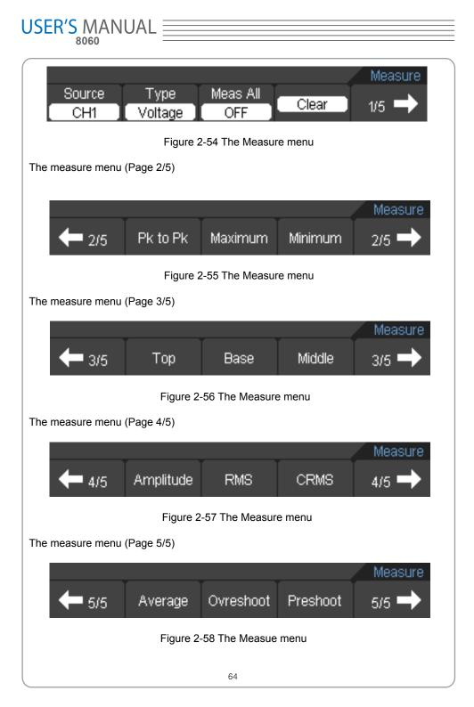
The scope meter provides 22auto measurements:Vpp,Vmax,Vmin,Vtop,Vmid,Vbase,Va mp, Vavg, Vrms,Vcrms, Overshoot, Preshoot, Freq, Period, Rise Time, Fall Time, +Width, -Width, +Duty, -Duty, Delay1->2↑, Delay1->2↓ (12 voltage and 10 time measurements).
