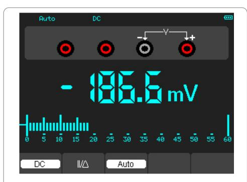
Figure 4-6 DC voltage Measurement
