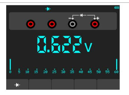
Figure 4-3 Diode Measurement
