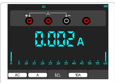
Figure 4-11 AC Current Measurement for 10A
