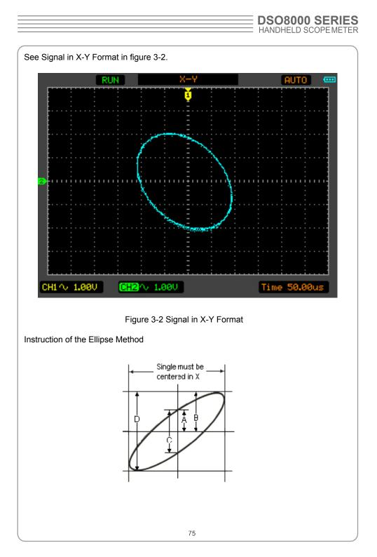
$Sin\theta = A/B$  or C/D, where  $\theta = phase shift$  (in degrees) between the two signals. From the formula above:
