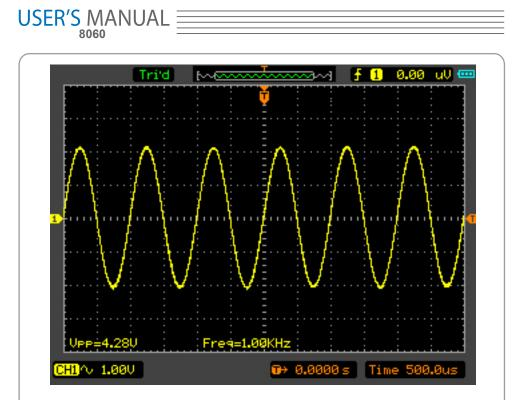
Figure 3-1 The Vpp and Freq measurement Window
