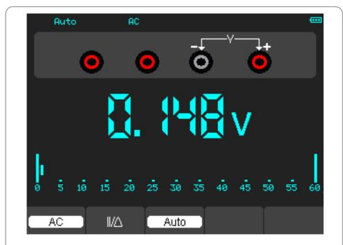
Figure 4-7 AC voltage Measurement
