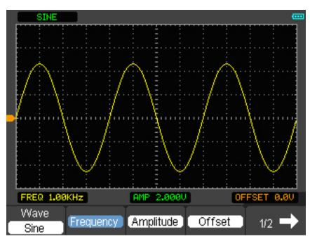
Press F1 to change the waveform to the sine waveform
