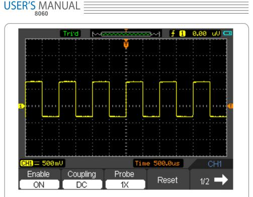
Figure 2-4 Waveform Display
