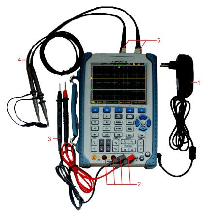
Figure 1-4 Input Connections
