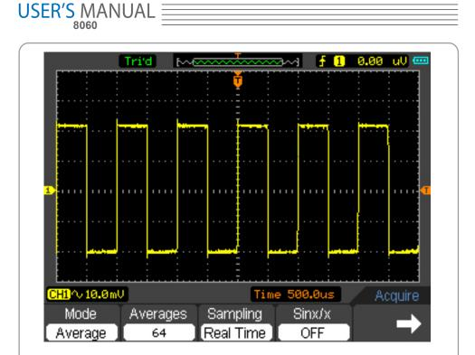
Figure 3-7 Signal afer reducing random noise
