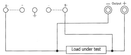
Attention: Disconnect the installed S- & S+ shorting wires when using the sampling connections.
