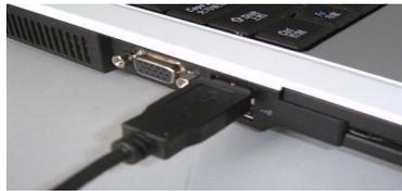
2. Connect the B-Type Plug of USB cable to DSO-2090 USB'S USB port.
