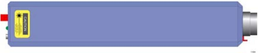
**Figure 7. Top view of laser showing the location of the “warning logotype” label for a Class II laser.**
