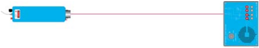
Figure 8. Class IIIa laser and laser beam aligned with an UT-Fiber Optics' audio laser receiver for demodulation of the laser beam's modulated signal and producing sound waves.
