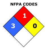
**Health and Safety:** The 8331 parts can ignite if the liquid is both heated and exposed to flames or sparks.
